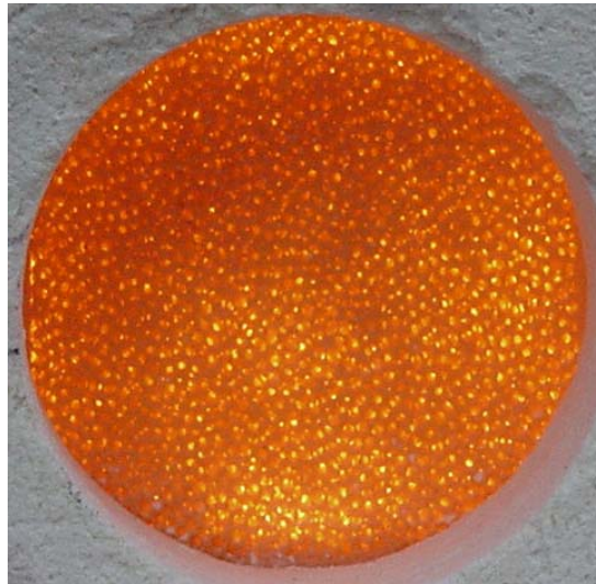
Figure 3 Oil flame inside of a ceramic radiant burner at BNL
